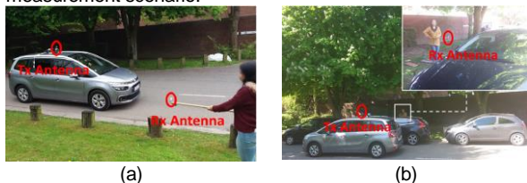
Fig. 1. Example of LoS (a) and NLoS (b) Measurements.
