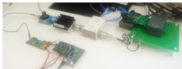
Fig. 2. Photograph of the global system: emitter and receiver (10.17 Mbits/s uplink and 3.39 Mbits/s downlink)
