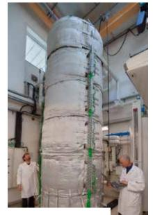
The first-ever tool for the study of granular material growth on the walls of the tank containing the material
