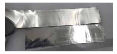
develop a pilot lamination machine that could reduce the thickness of the lithium-metal layer—currently 50 microns—by half. A thinner layer would increase the amount of energy that can be held by an equivalent volume.
