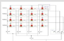
High-density SOT-MRAM memory array based on a single transistor
