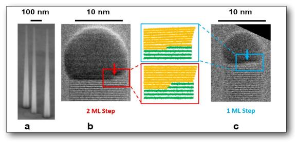
Figure: (a) ZnTe nanowires grown in MBE cluster; (b) Nanomax image showing the gold seed at the top of the ZnTe nanowire, with a two-monolayer step at the interface; the step (indicated by the arrow) propagates from right to left; (c) idem, with a one-monolayer step. The schemes in-between display the Au atomic planes (in yellow) and the ZnTe planes (in green) for the two configurations.
