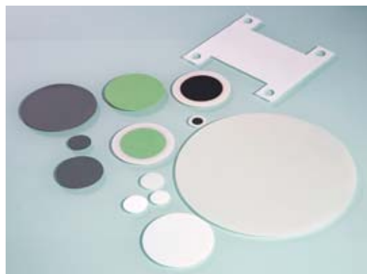
Planar HTE components: electrolytes, electrolyte-supported cells, and electrode-supported cells.
