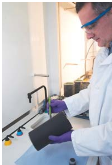
Tubular HTE cells. Development work on 600-cm 2 cells, for an innovative coaxial architecture. Electrode deposition by coating.
