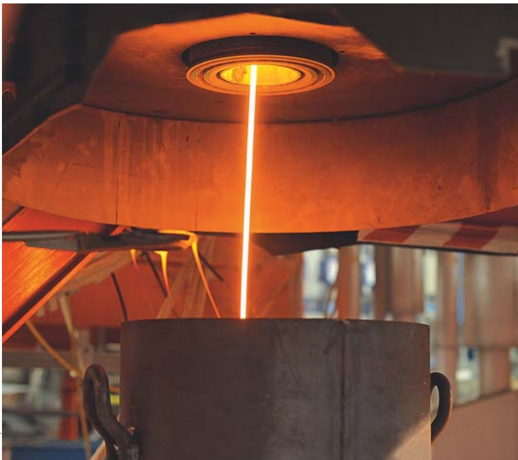
Glass pouring from the Upgradeable Vitrification Prototype (PEV: Prototype évolutif de vitrification), fitted with a cold-crucible furnace, set up at CEA/Valrhô-Marcoule.
