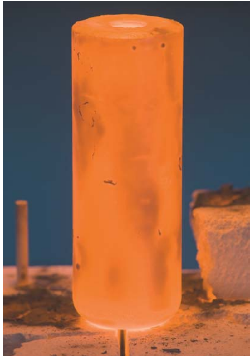
Cladding (billet), raised to a high temperature – about 1,100 °C – containing ODS powder. The billet is ready to undergo hot extrusion, using a press.
