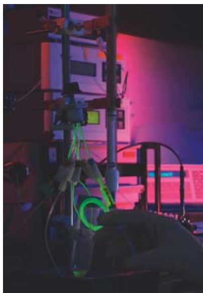
A small soil column, used for the investigation of nanoparticle migration, by means of fluorescent nanotracers.
