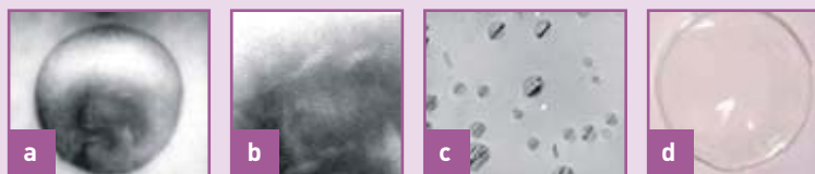
Figure 3. Detail micrographs of the (mesoporous) nanostructure of a composite sol-gel matrix.
