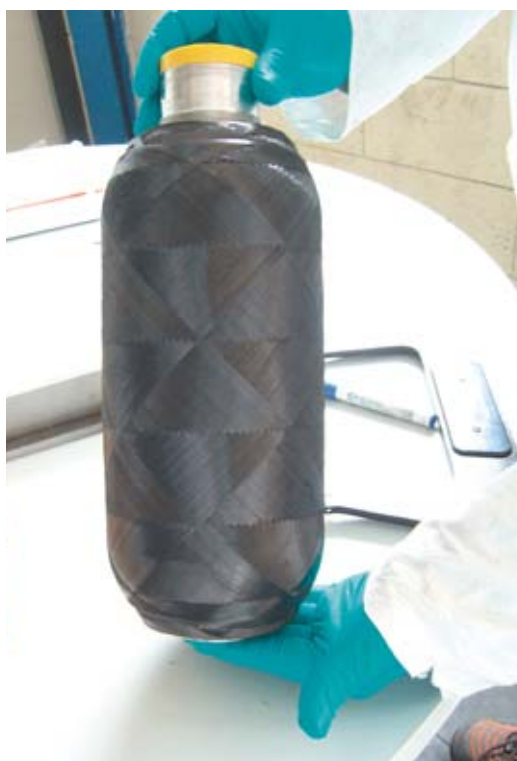
Fabrication of a composite structure by filament winding, from continuous carbon fibers.
