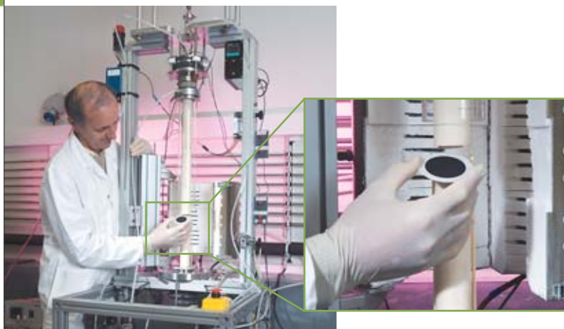
A high-temperature electrolyzer (HTE) cell being mounted in a test bench, serving to determine cell performance, and durability.
