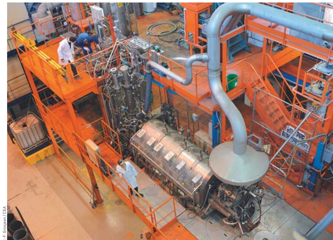
General view of the Upgradeable Vitrification Prototype (PEV: Prototype évolutif de vitrification), fitted with a cold-crucible furnace, set up at CEA/Valrhô-Marcoule.
