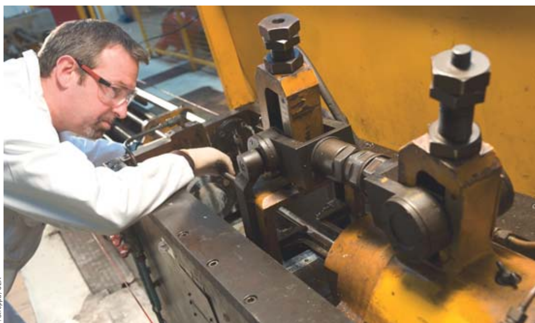
The cold rolling step, for ODS-alloy tubes, has the purpose of shaping the extruded blank, to obtain thin tubes, exhibiting the desired geometry.
