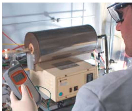
Experimental synthesis of carbon nanotubes by chemical vapor deposition (CVD).
