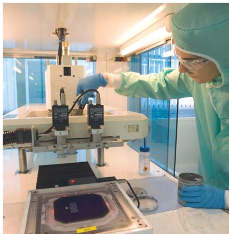
Screen-printing the metal contacts onto a silicon photovoltaic cell.
