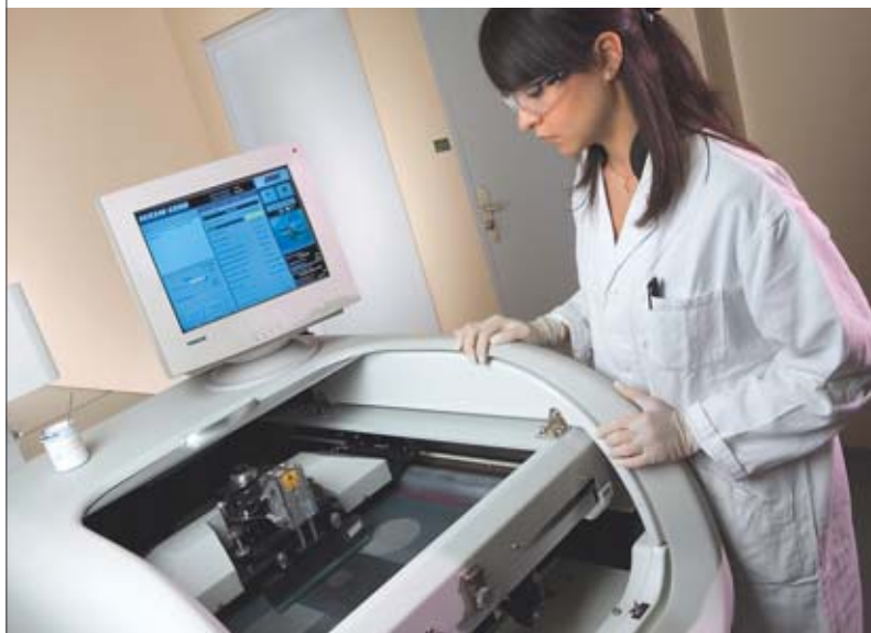
A screen-printing bench, being used for the application of a ceramic ink.
