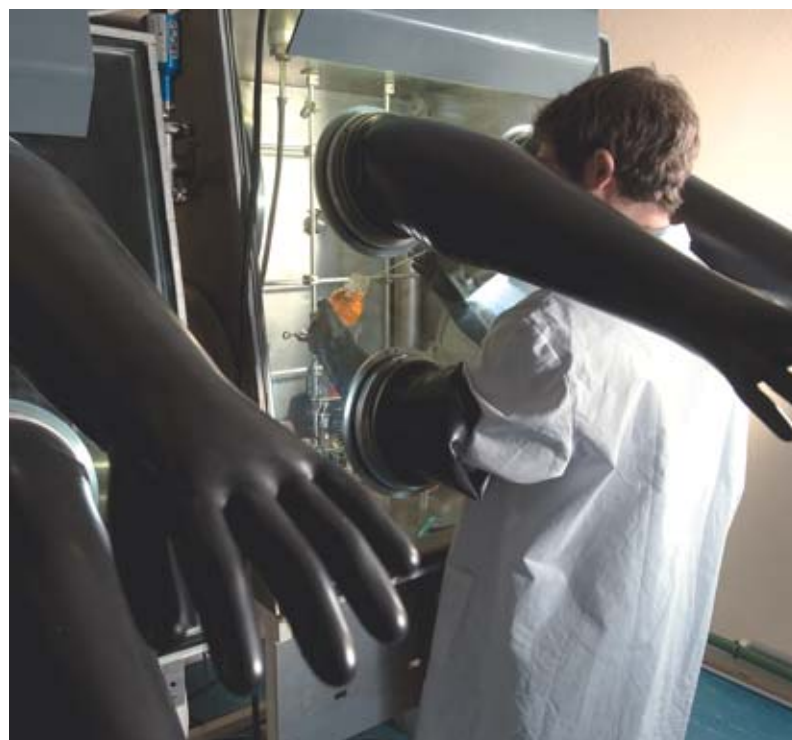
Covalent grafting of ultrathin lubricating films sometimes calls for operations to be carried out in glovebox conditions, to analyze the effects of atmospheric pollutants.
