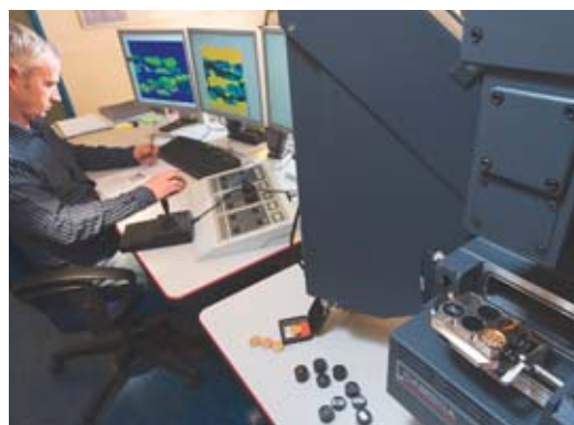
General view of the “Castaing” electron microprobe, which makes it possible to quantify, in particular, the distribution, at the micron scale, of added elements, and impurities, within fuel claddings.
