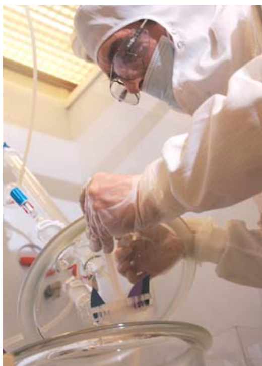
A technician, operating in a white room, at work on a dedicated chemical reactor, used for the collective silanization of silicon wafers, or glass plates used for the preparation of DNA chips, or laboratories-on-a-chip.
