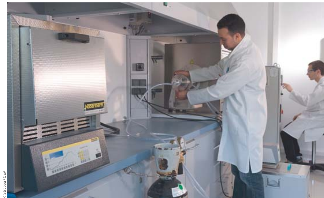
Synthesis furnaces, used for the structuring agent removal step (see Figure in Box).
