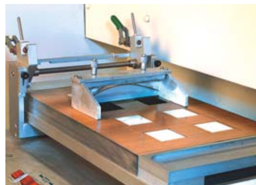
Coating bench for PEM fuel-cell active layers. A membrane is being coated with an ink consisting of platinum/carbon, and electrolyte particles.
