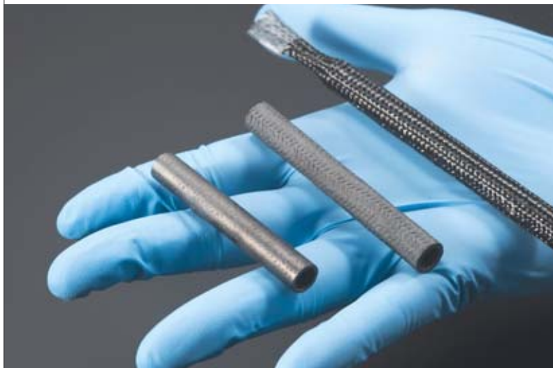
Figure 4. A silicon-carbide braid (at right), seen after densification (middle), and after the machining operation to remove the outer sacrificial layer (left).
