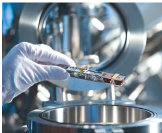
X-ray photoelectron spectroscopy (XPS): positioning a sample holder in the entrance bay of the spectrometer.
