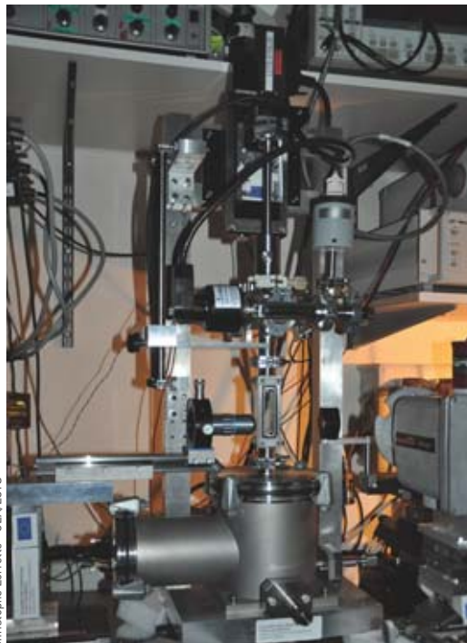
A rig used to measure the thermal conductivity of microcomposites, set up at the Thermostructural Composites Laboratory.
