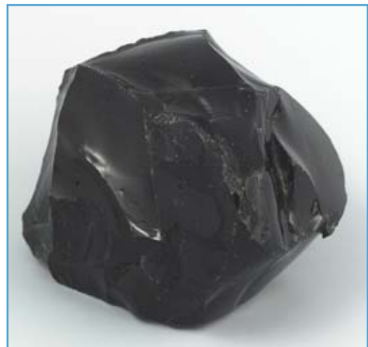
A block of containment glass (R7T7 glass).
