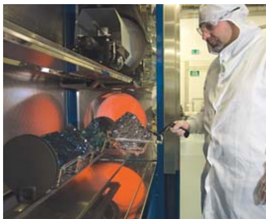
Boron and phosphorus diffusion furnace, used for doping purposes (Restaure platform-INES).
