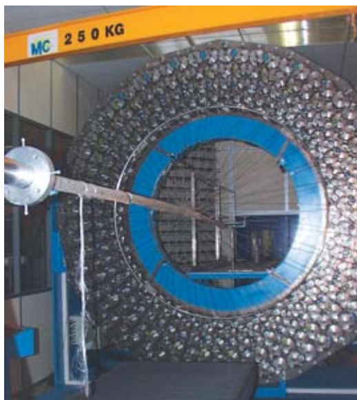
Braiding machine, serving for the fabrication of triaxial braids.
