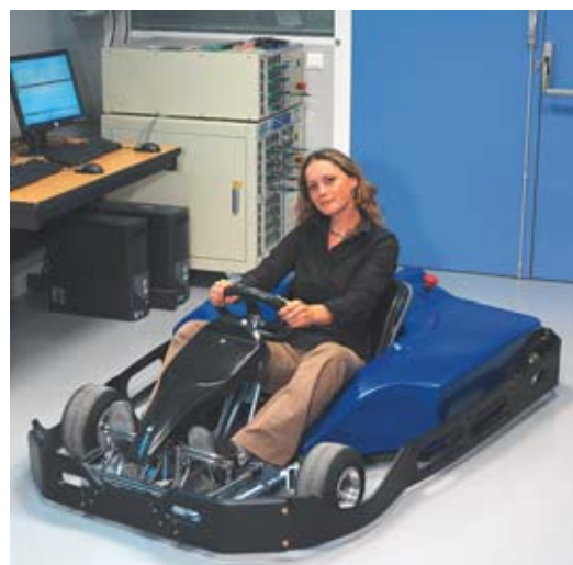
Prototype go-kart, powered by a lithium storage battery.
