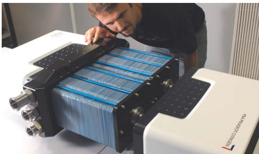
The GENEPAC (Générateur électrique à pile à combustible: Fuel-Cell Electric Generator) fuel cell, developed by CEA, in partnership with PSA Peugeot Citroën, for a forthcoming automotive application.
