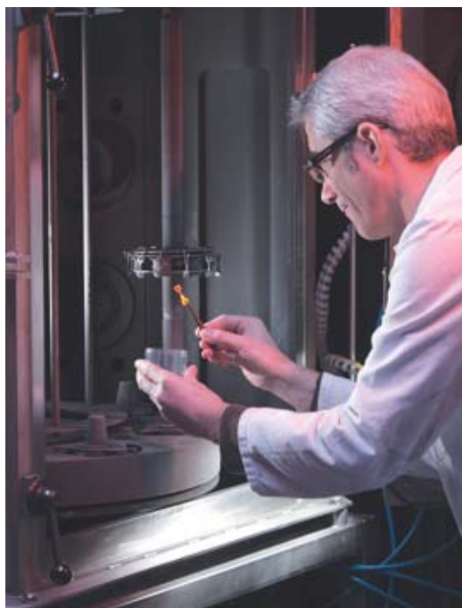
The deposition chamber of the vacuum arc evaporation reactor, featuring a substrate holder able to move about three rotational axes.
