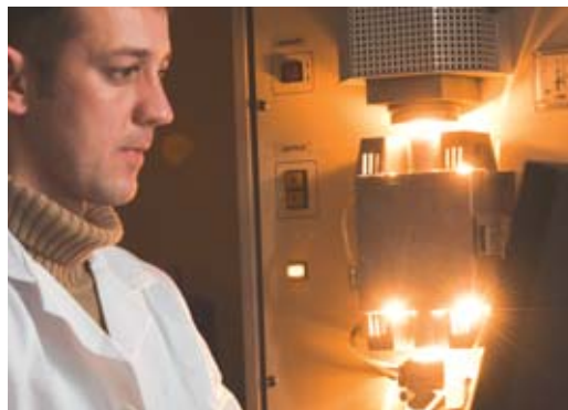
Quench dilatometry test being carried out on a cladding sample, subjected to dynamic heating, and subsequent cooling ramp conditions (up to 100 °C/s).
