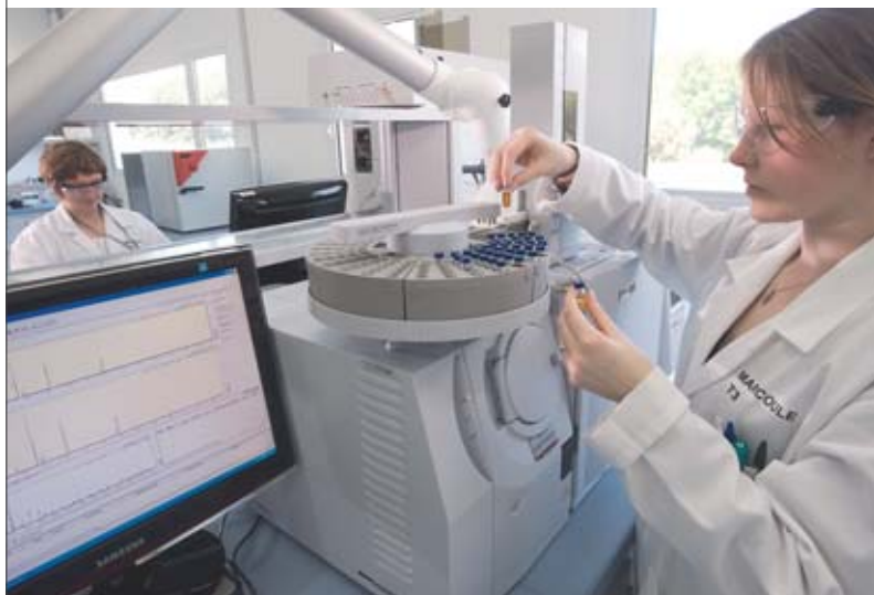
A gas chromatograph, coupled to a mass spectrometer (GC-MS), serving to monitor the synthesis of organic functional grafts.
