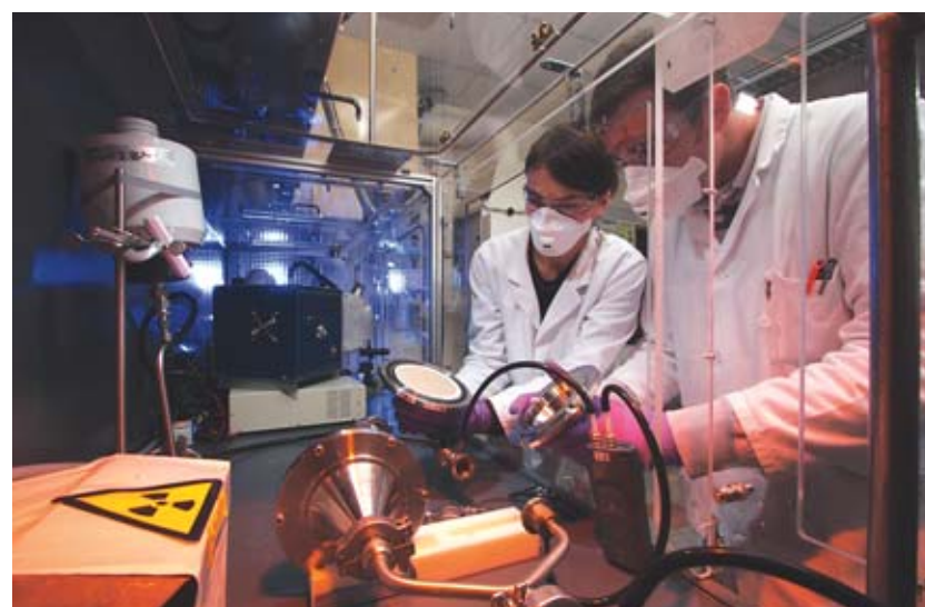
A dedicated glovebox, used for nanosafety studies. Shown here, a test on clothing to be worn by operators involved in the production, and handling of nanopowders, and nano-objects.
