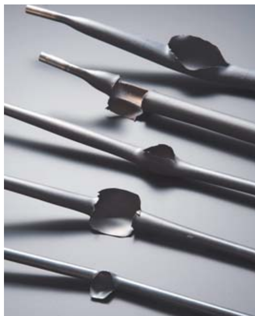
Cladding samples, after undergoing burst testing in high-temperature accident conditions in the “EDGAR” facility.
