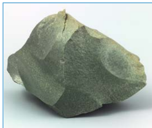
A block of glass–crystalline material, used for the containment of old solutions yielded by the treatment of \text{UMo} fuels from UNGG reactors.
