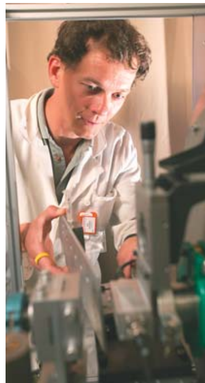
Small-angle X-ray scattering apparatus, being used to characterize nanoparticle size, shape, and concentration.
