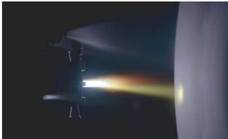
Fabrication of nanostructured coatings by thermal spraying.
