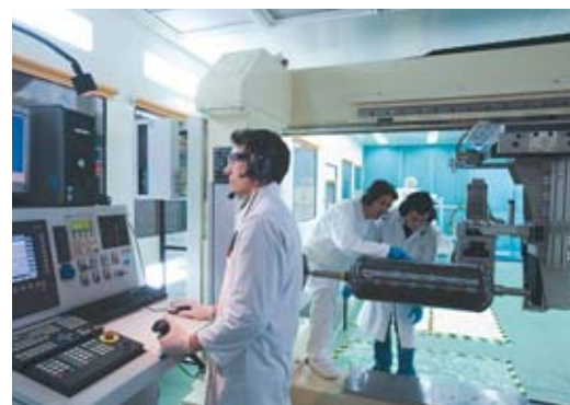
Fabrication of a composite structure by filament winding, from continuous carbon fibers.
