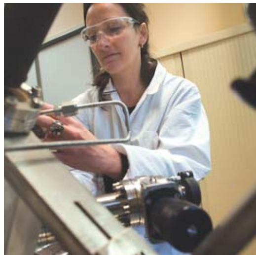
Diamond growth being carried out in a microwave-plasma-assisted chemical vapor deposition (MPCVD) reactor.
