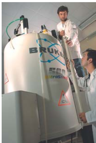
The magnet of the high-magnetic-field solid-state NMR spectrometer used for the purposes of investigating the structure of materials. The resonance frequency for the hydrogen nucleus, i.e. the proton, stands at 500 MHz in this magnet.
