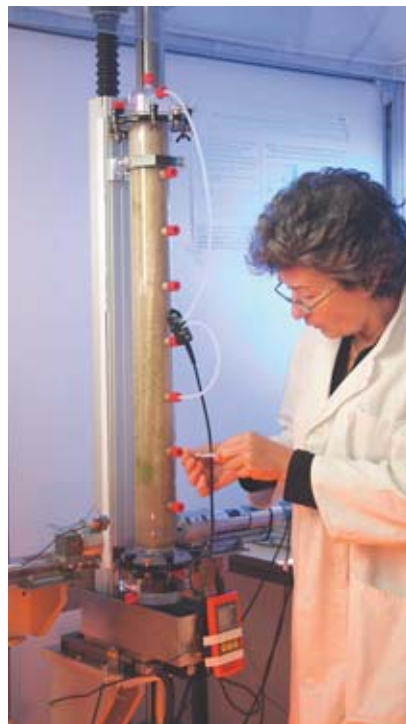
Investigation of nanoparticle migration in soils, to ensure the preservation of potable water resources. The soil column is positioned on a gamma-ray measurement bench, to record soil water content on a continuous basis.
