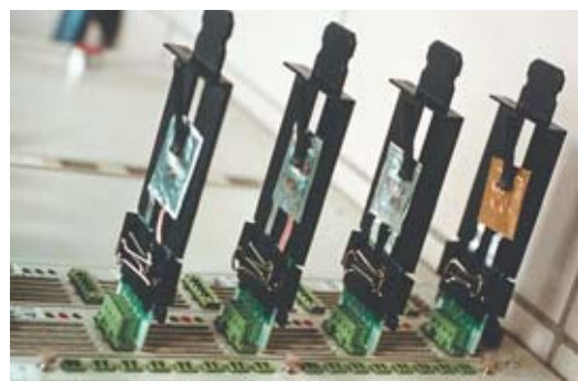
Cycling benches for lithium systems, ranging from a button cell to a mini-battery. Button cells are used for materials testing; the flat units are prototype lithium-polymer mini-batteries, intended for integration into smart cards.
