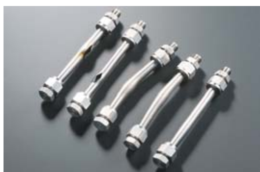
Testing apparatus used for cladding burst tests from internal pressure in nominal conditions (around 350 °C), and picture of cladding segments subsequent to testing.
