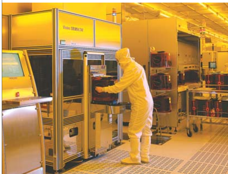
An operator loading the electron-beam exposure system. This equipment allows patterns smaller than 11 nm to be traced onto 300-mm-diameter silicon wafers.
