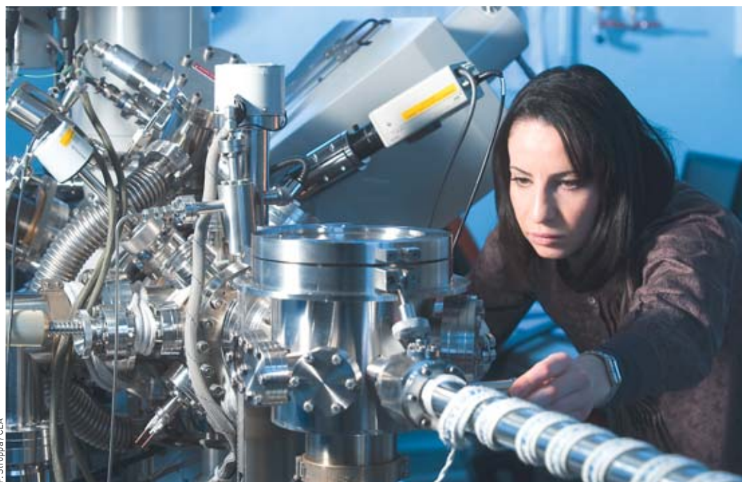
X-ray photoelectron spectrometry (XPS): positioning a sample holder in the analysis chamber.
