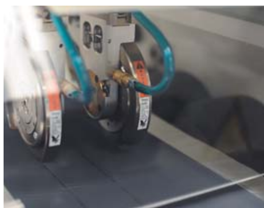
Electrode undergoing slitting (cutting).
