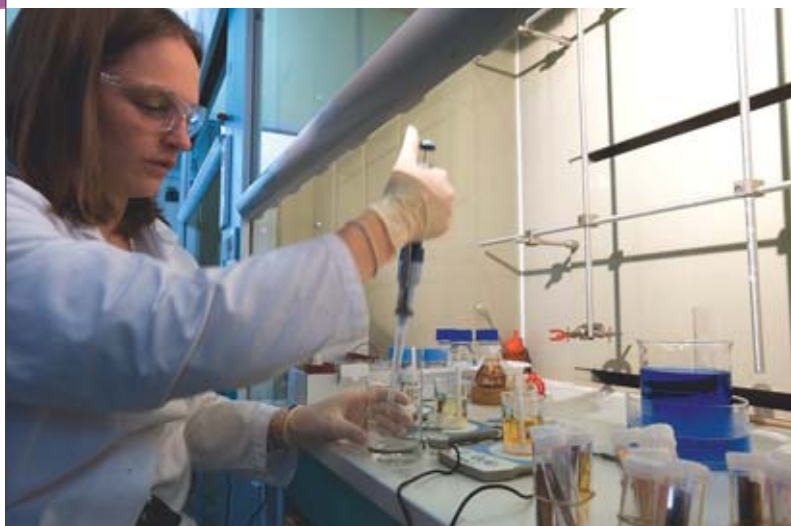
Covalent chemical grafting by the GraftFast™ process: preparation of the reactive mixture.
