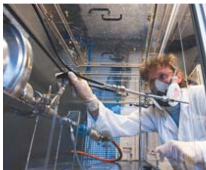
Setting up an experiment serving to test the imperviousness to nanoparticles of personal protective equipment (masks, gloves), as part of the European NanoSafe project.
