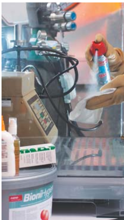
Setting up a nanoparticle release test for nanoproducts in general use (polymers, fabrics...).
