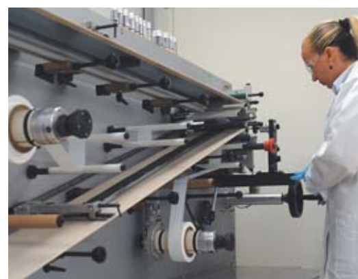
Spooling of electrodes (both positive, and negative), and separators.
