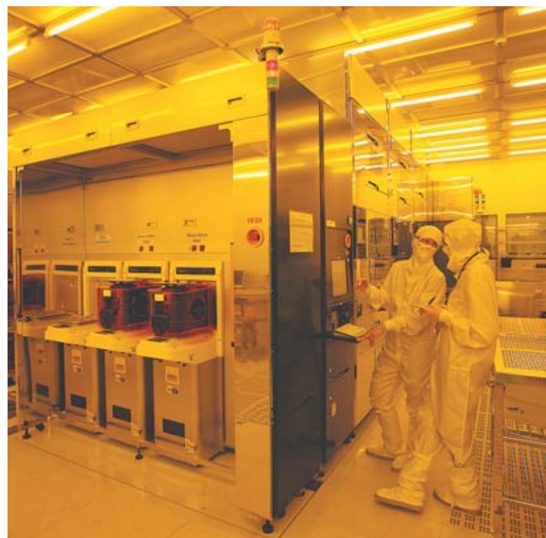
Operators standing in the photolithography zone, in front of the exposure system used for 300-mm wafers.
