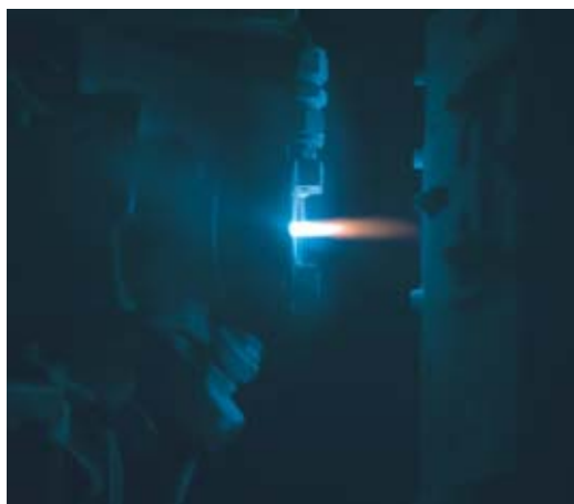
Suspension plasma spraying of ceramic nanopowders, carried out at CEA/Le Ripault.
