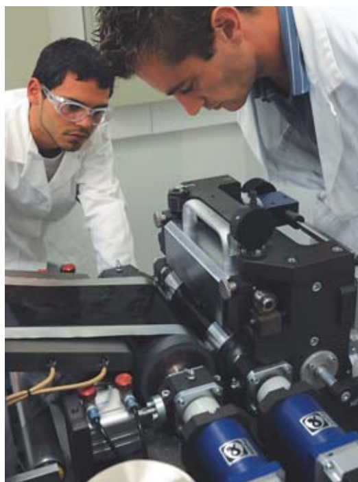
Electrode undergoing coating in a small pilot bench.
