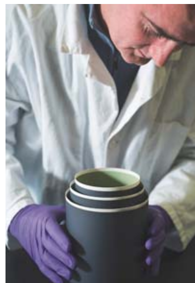
Tubular HTE cells. Development work on 600-cm 2 cells, for an innovative coaxial architecture. Electrode deposition by coating.
