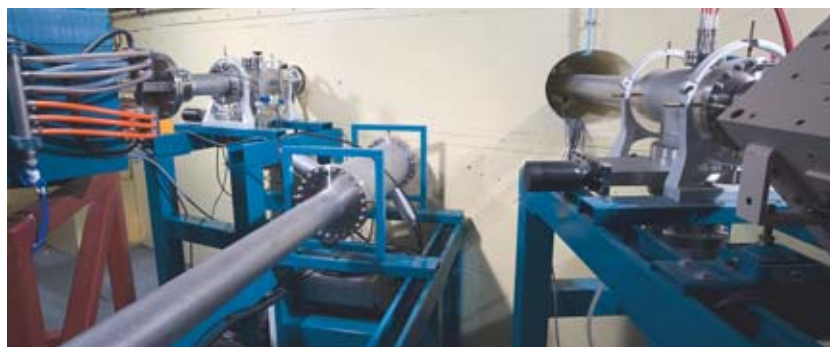
The beamlines from JAPET (left), YVETTE (center), and EPIMETHEE (right), converging onto the triple-beam experiment chamber, located behind the wall.
