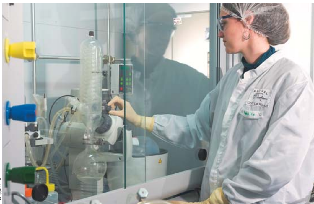
An operator setting up a nanoparticle synthesis operation – taking place in a fume hood – by the sol–gel process, in a rotary evaporator.
