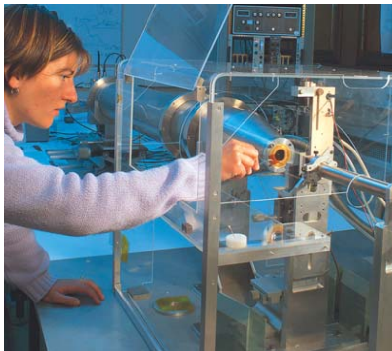
A small-angle X-ray scattering camera, used for the investigation of fuel-cell membrane structures, at the nanometer scale.
