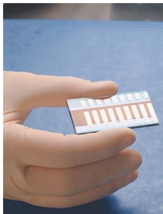
A new type of photovoltaic cell is being developed, using conducting organic polymers, deposited onto glass substrates.
