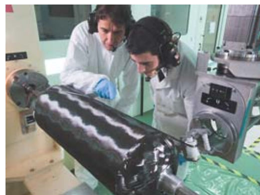
The stacking of hoop, and spiral plies, resulting in the fabrication of the tank's structural composite shell.
