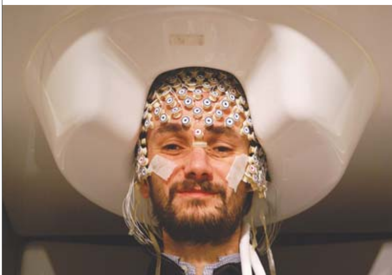
Volunteer installed in the MEG system and wearing an electroencephalography cap. The EEG and MEG enable information transfers through the brain to be monitored millisecond by millisecond.
