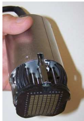
Sonde flexible multi-éléments
