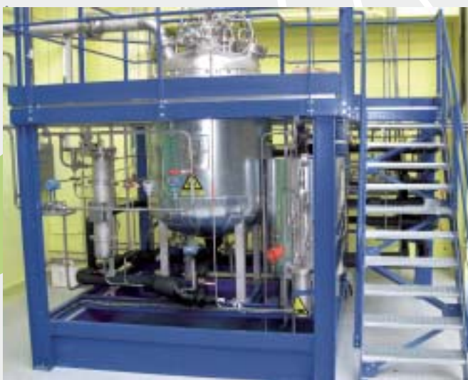
MININANET: CEA facility for sodium hydrolysis studies.
