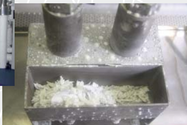
Carbonation of sodium retention (mock-up of Rapsodie).
