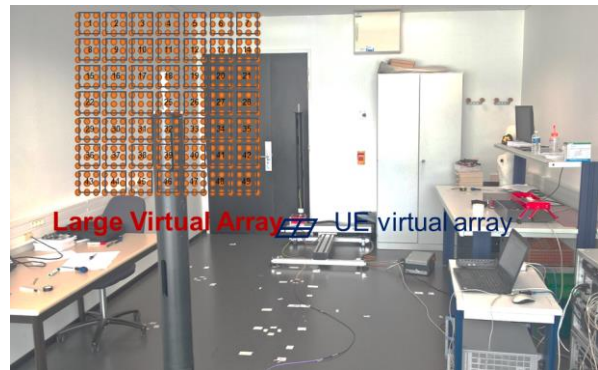
Fig. 1: Indoor mmwave channel measurement campaign employing large array, and repartition in sub-arrays.
