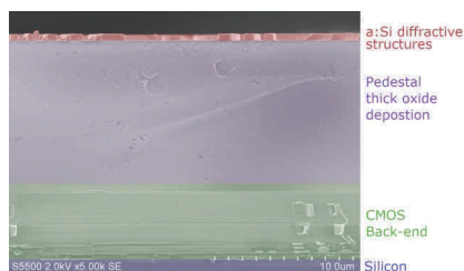
Fig. 1. Vertical cross-section of optical spacer and a:Si microlens processed on CMOS wafer
