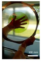
Figure 2: 200 nm ultra-thin silicon film transfer to a flexible substrate [3].
