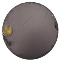
Figure 1: Φ=148 mm Cd<sub>1-y</sub>Zn<sub>y</sub>Te (lapped) crystal
