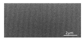
Figure 1: Seamless stitching of 4 fields (CD = 50 nm
