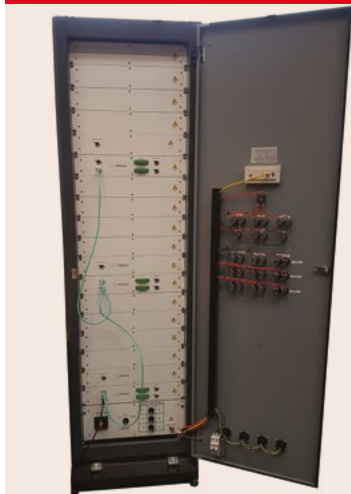
▲ 30 kW stationary storage system with Sigma Cells all-in-one charger, inverter, and BMS
