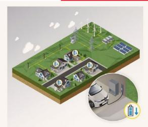
When the energy supply is lower than the demand, vehicle charging stops. The plugged-in vehicles can then return electricity into the grid. This is called bidirectional charging, or Vehicle to Grid.
