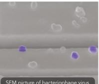
SEM picture of bacteriophage virus Γ5 capsids (false color) deposited onto the active area of a nano-resonator after mass measurement.
