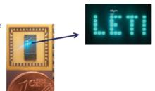
Key innovations include micro-structuration of LED arrays (10  $\mu$ m pitches or smaller) with high efficiency, and 3D heterogeneous integration (hybridization) of LED arrays on CMOS circuits.
