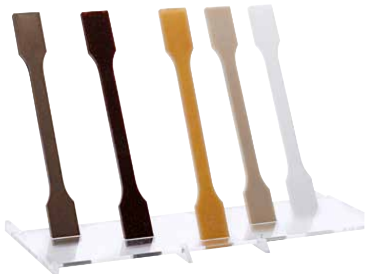
Bio-based material test samples. The colored samples are natural fibers (linen, hemp, coir); the white sample is a polymer fiber.
