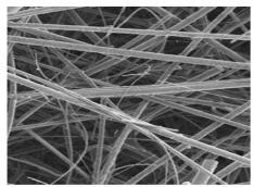
Fibrous filter as seen through a microscope
