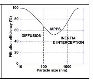
Finally, the smaller the particles and the higher the filtration efficiency by diffusion phenomena are.
