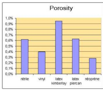
The porosity to helium (~0.3 nm) seems specific to a type of material.
