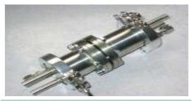
The "through diffusion method" derivates from standard NF EN ISO 6529 and NF EN 374 uses a diffusion cell in which a constant particle concentration is imposed in the upper flow part. Diffusion coefficients are calculated from the measurement of nanoparticle flowing in the down flow part of the cell.
