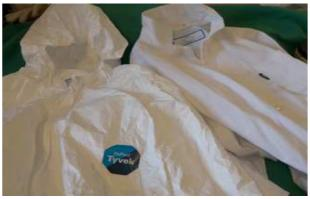
Tests performed with graphite nanoparticles centred at 40 nm and 80 nm showed that high density polyethylene textile (Tyvek® type) seems to be better than cotton and polypropylene.
