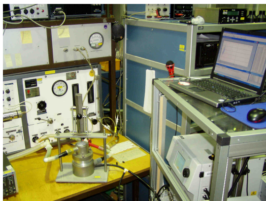
Setup for penetration tests of RPE against salt aerosol BGIA DGUV photograph
