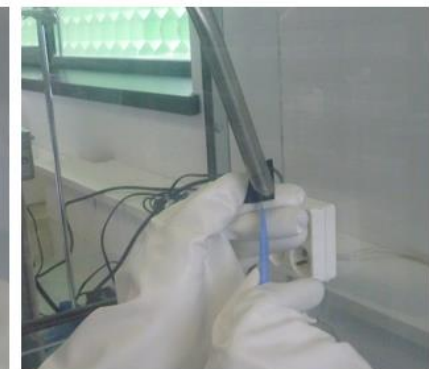
Scraping on CNT sample
