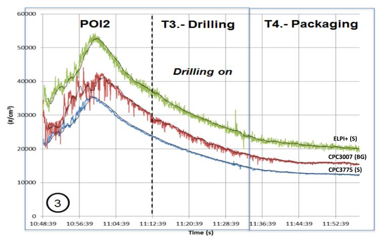
Raw time series of PNC as captured at source and background during drilling and packaging nano-TiO<sub>2</sub> enabled steel tablets. Temporal background signal overrides the potential contribution of NPs release during mechanical processing (POI2: Period of Inactivity 2)
