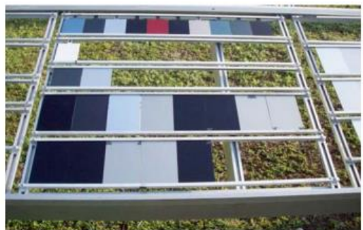
FIG. 1 Suitably Mounted Specimens in a Frame
