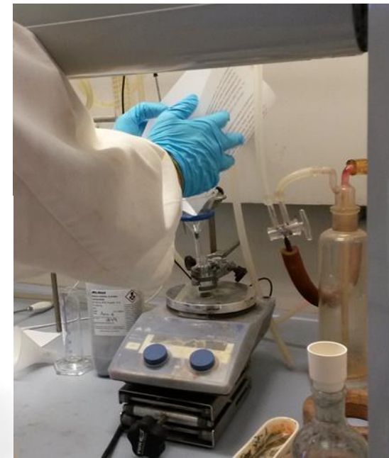
Scratching crucible to remove all residues
