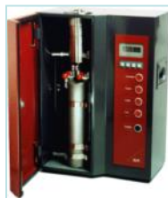
ELPI Electrical Low Pressure Impactor
