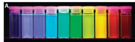
Fig.: Size-dependent colour of QDs and their emission spectra in Zrazhevskiy P., 2009: DOI: 10.1039/b915139g
