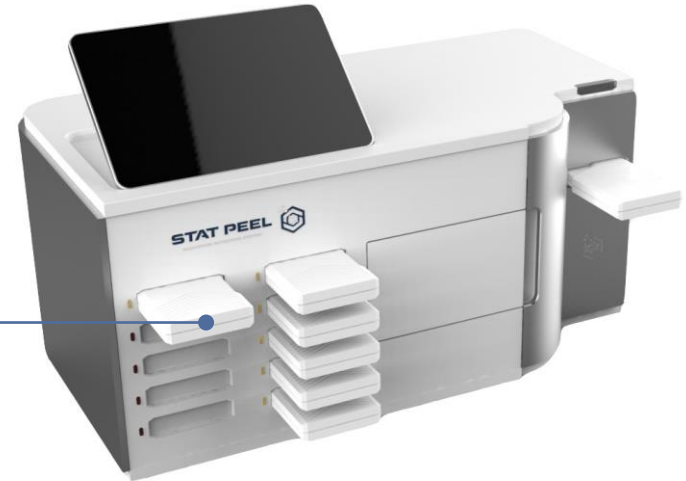
Reader with filtration slide exchange, badge charging station and data-management.
