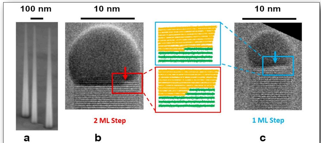
**Figure:** (a) ZnTe nanowires grown in MBE cluster; (b) Nanomax image showing the gold seed at the top of the ZnTe nanowire, with a two-monolayer step at the interface; the step (indicated by the arrow) propagates from right to left; (c) idem, with a one-monolayer step. The schemes in-between display the Au atomic planes (in yellow) and the ZnTe planes (in green) for the two configurations.
