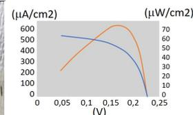
Polarization curve of the fuel cell after explantation (blue: surface current - left axis, orange: surface power - right axis).
