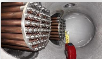
Figure 1: Inside view of heat exchanger with copper tube bundles.
