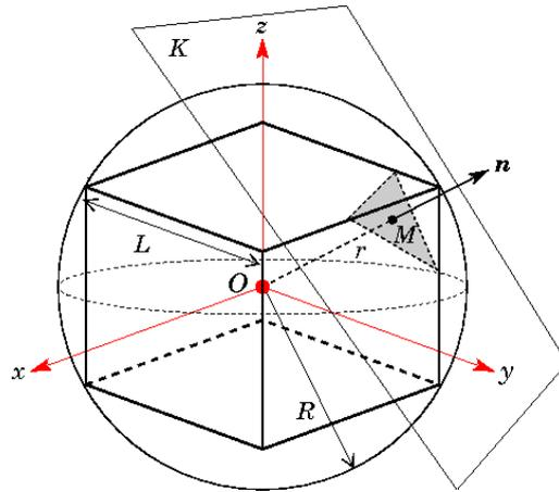
*Fig. 3. Poisson tessellation of a cube of side  $L$  in dimension  $d = 3$ : drawing a random plane  $K$ . The circumscribed sphere has a radius  $R = \sqrt{3} L / 2$ . The point  $M$  is defined by  $OM = r n$ , where  $r$  is drawn uniformly over the interval  $[-R; R]$  and the normal vector  $n$  of each hyperplane is drawn from an arbitrary distribution  $H(n)$ . The plane orthogonal to the vector  $n$  and passing through  $OM$  is the desired random plane  $K$  [3].*
