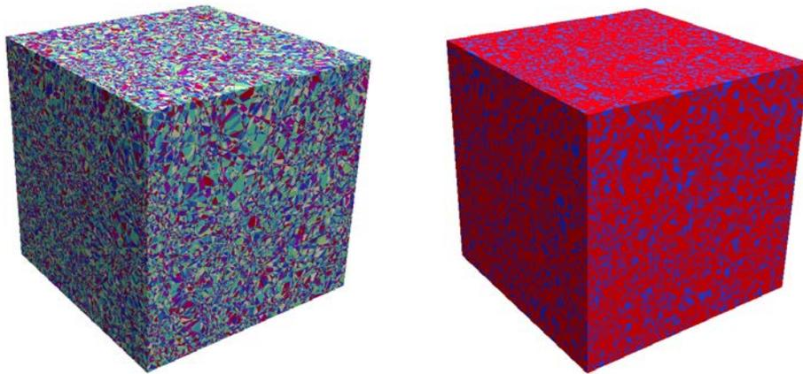
*Fig. 1 et 2. Left: Example of realization of a homogeneous and isotropic random Poisson tessellation, in three dimensions, created by using the generator of random geometries developed at CEA [3]. Right: The same realization after applying a binary coloring procedure for the polyhedra (probability of red 75% and blue 25%). These tessellations are spatially homogeneous, their statistical properties being the same at any point in space.*
