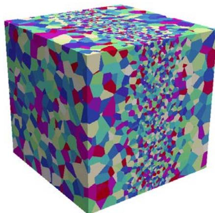
*Fig. 5. Example of realization of a three-dimensional non-homogeneous random Voronoi tessellation, with spatial gradient along an axis (the density of the tessellation is smaller at the edges and larger at the center of the volume), created from recent developments in the random geometry generator developed at CEA [10].*
