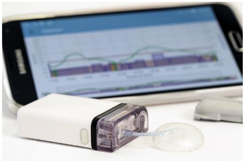
The startup Diabeloop is developing a portable artificial pancreas that combines a continuous glucose monitor, an insulin pump and a smartphone that hosts a personalized algorithm. © Pierre JACQUET/CEA
