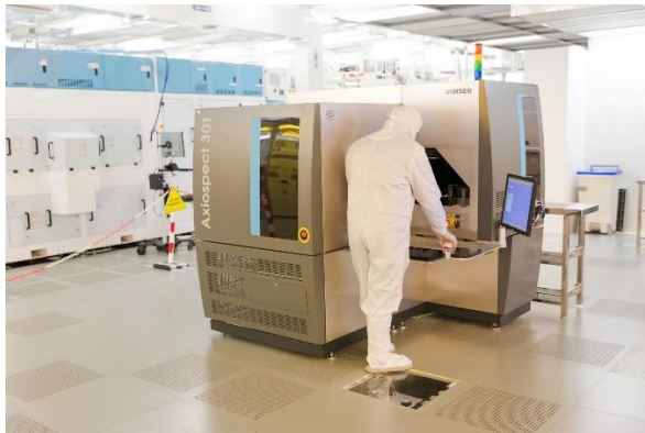
CEA-Leti clean room: 300-mm high-magnification inspection station. © Pierre JAYET/CEA.
