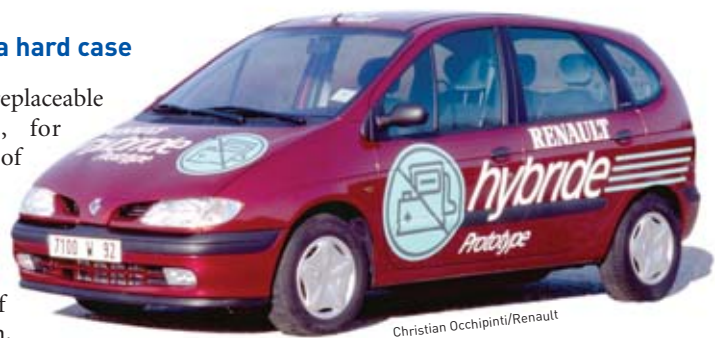
Hybrid vehicle of the Scenic type, built by Renault, powered by both a heat engine and electric batteries. This formula represents a likely step in the evolution to automobiles powered, in the longer term, by hydrogen-fed fuel cells.
