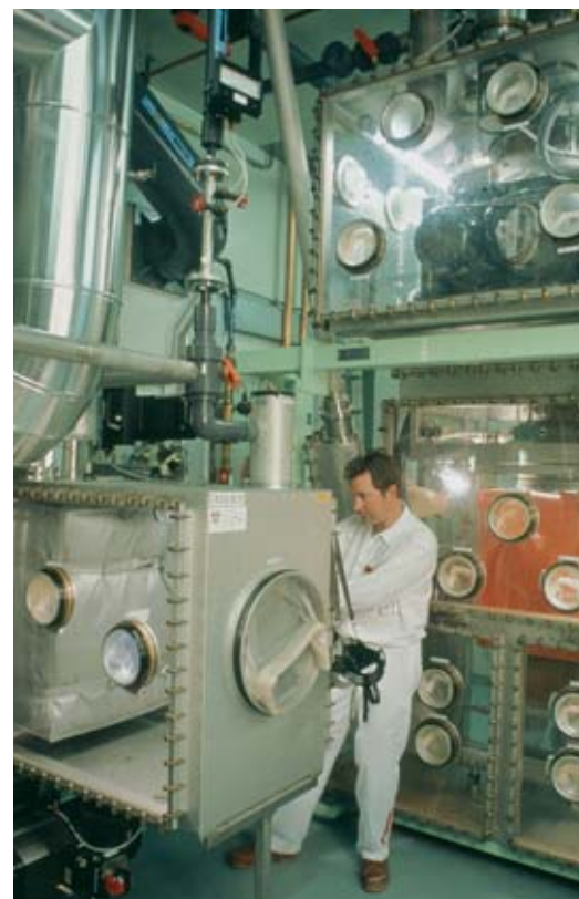
Alpha incinerator for the processing of technological waste from the Valduc center (Côte-d'Or département, Eastern France) of CEA's Military Applications Division.
