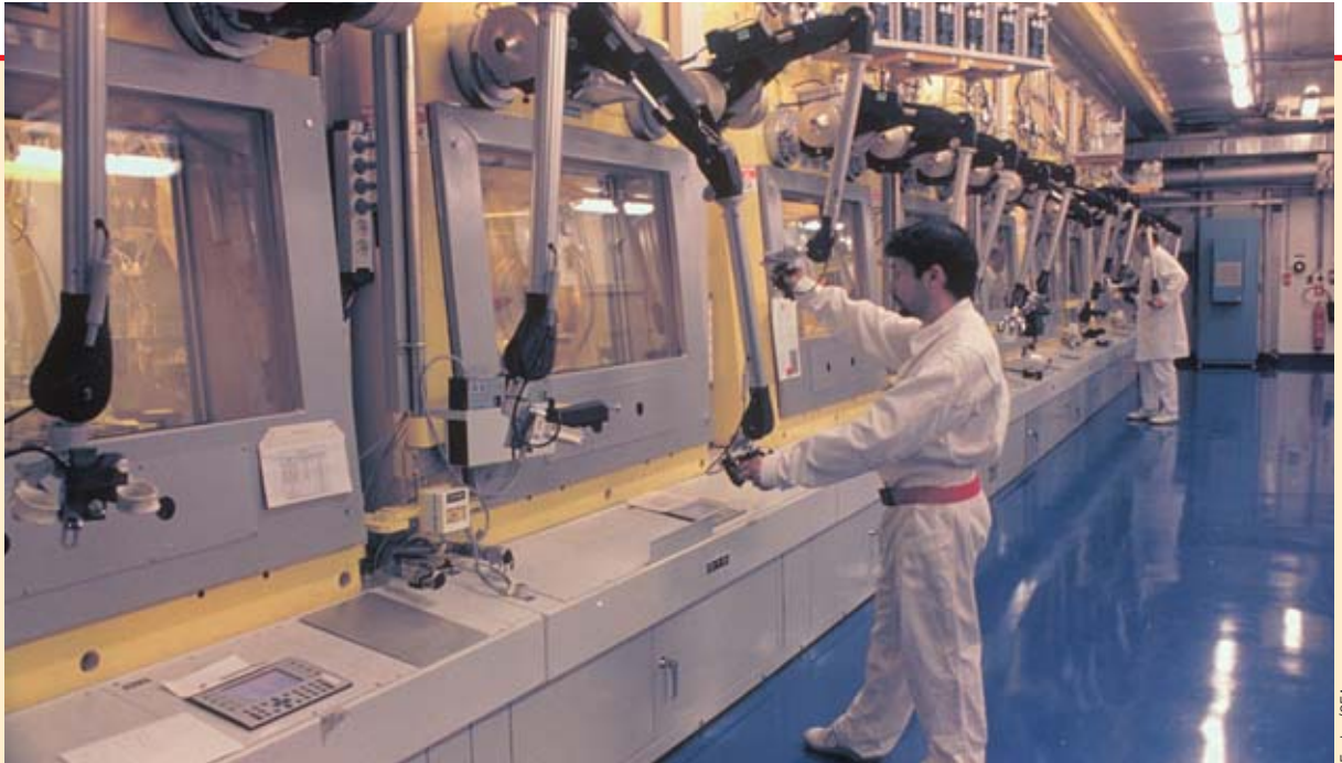
Technicians operating remote handling equipment on a line at the Atalante facility at CEA Marcoule. The shielding of the lines stops radiation. The operators wear personal dosimeters to monitor the efficacy of the protection.
