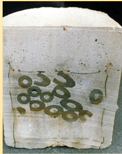
Example of waste embedded in a concrete matrix.
