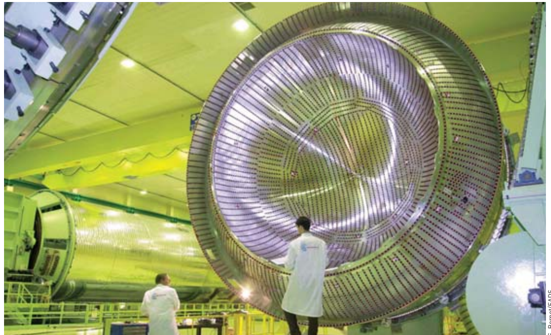
Cryogenic stages of the Ariane 5 space launcher being welded at Cryospace [ESC-A upper stage in the foreground, EPC main stage behind]. Space propulsion, while quantitatively limited, represents an initial industrial use of hydrogen as an energy carrier.
