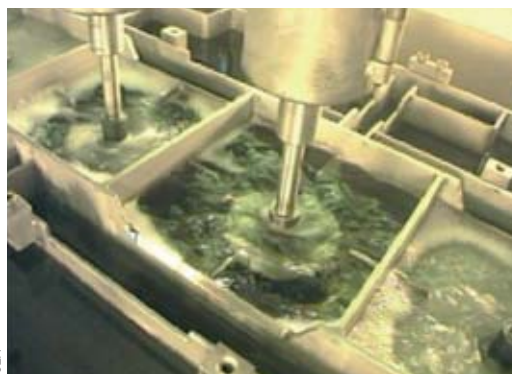
Decontamination of tanks through coupled use of surfactant solutions in an acid medium and mechanical agitation during cleanup of APM (Atelier pilote de Marcoule: Marcoule Pilot Workshop).
