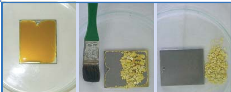
Figure 2. Decontamination by means of a vacuumable cerium gel.
