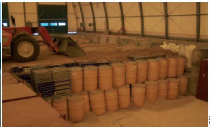
At the Morvilliers Disposal Center, VLLW waste is positioned in pits, shielded from rain by mobile roofs.
