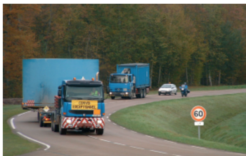
Transporting vessel heads to the Soulaines Disposal Center. Operational solutions are provided for large waste items.
