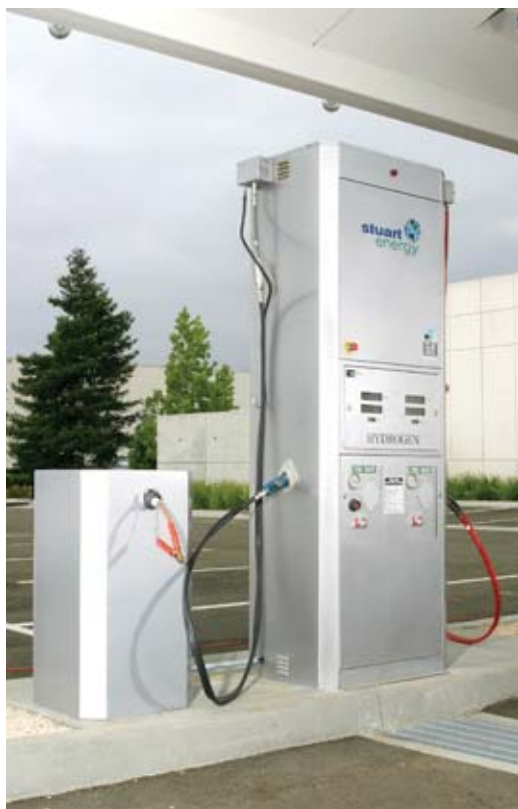
Hydrogen dispenser module fed by an electrolysis unit.
