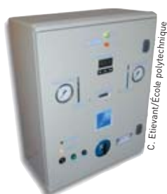
Prototype solid-polymer-membrane electrolyser for hydrogen and oxygen generation, developed in collaboration with the French École polytechnique.
