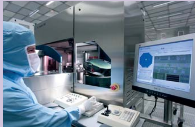
Visual inspection of integrated circuits in the Crolles2 Alliance facilities.
