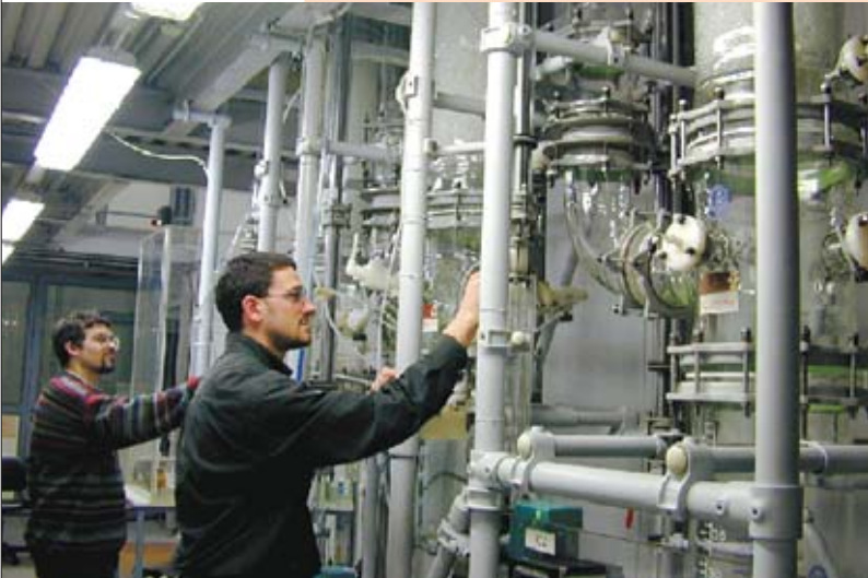
Chemical extraction of germanium 71 from the gallium-chloride target solution, prior to conversion of the germanium chloride into germanium hydride, during the Gallex experiment.
