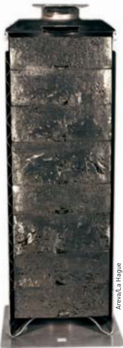
Cross-section view of a standard compacted waste container (CSD-C), showing the stack of pellets of compacted structural waste (hulls and end-caps) or technological waste.
