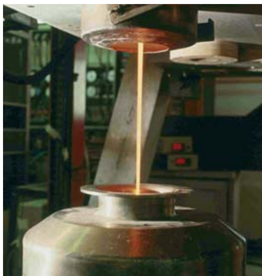
Glass being cast in the Marcoule Vitrification Workshop (AVM: Atelier de vitrification de Marcoule).
