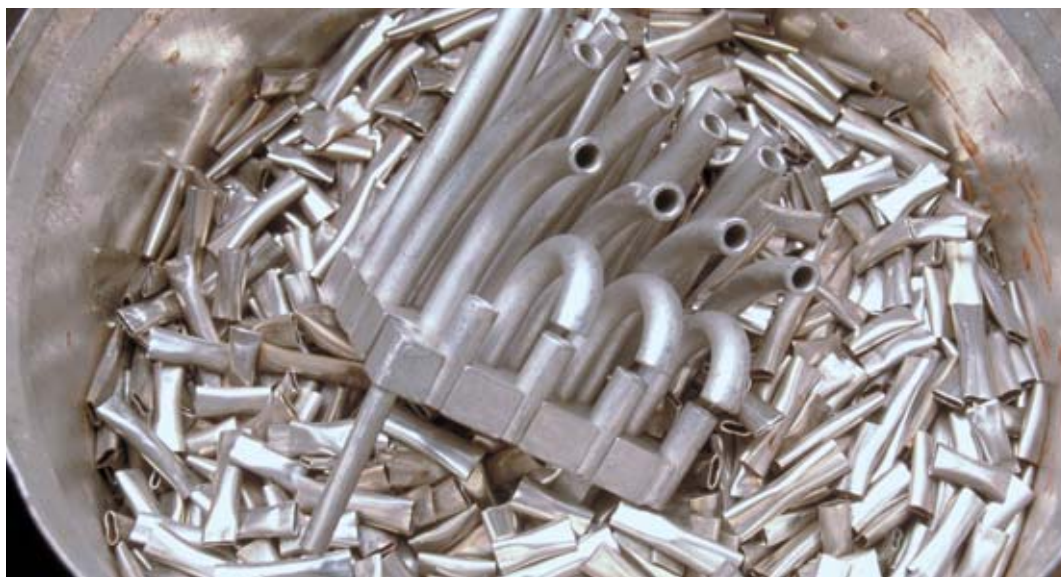
Compaction of hulls and end-caps , waste from the structures of spent fuel assemblies, has taken the place of cementation, thus yielding a reduction in volume by a factor 4.
