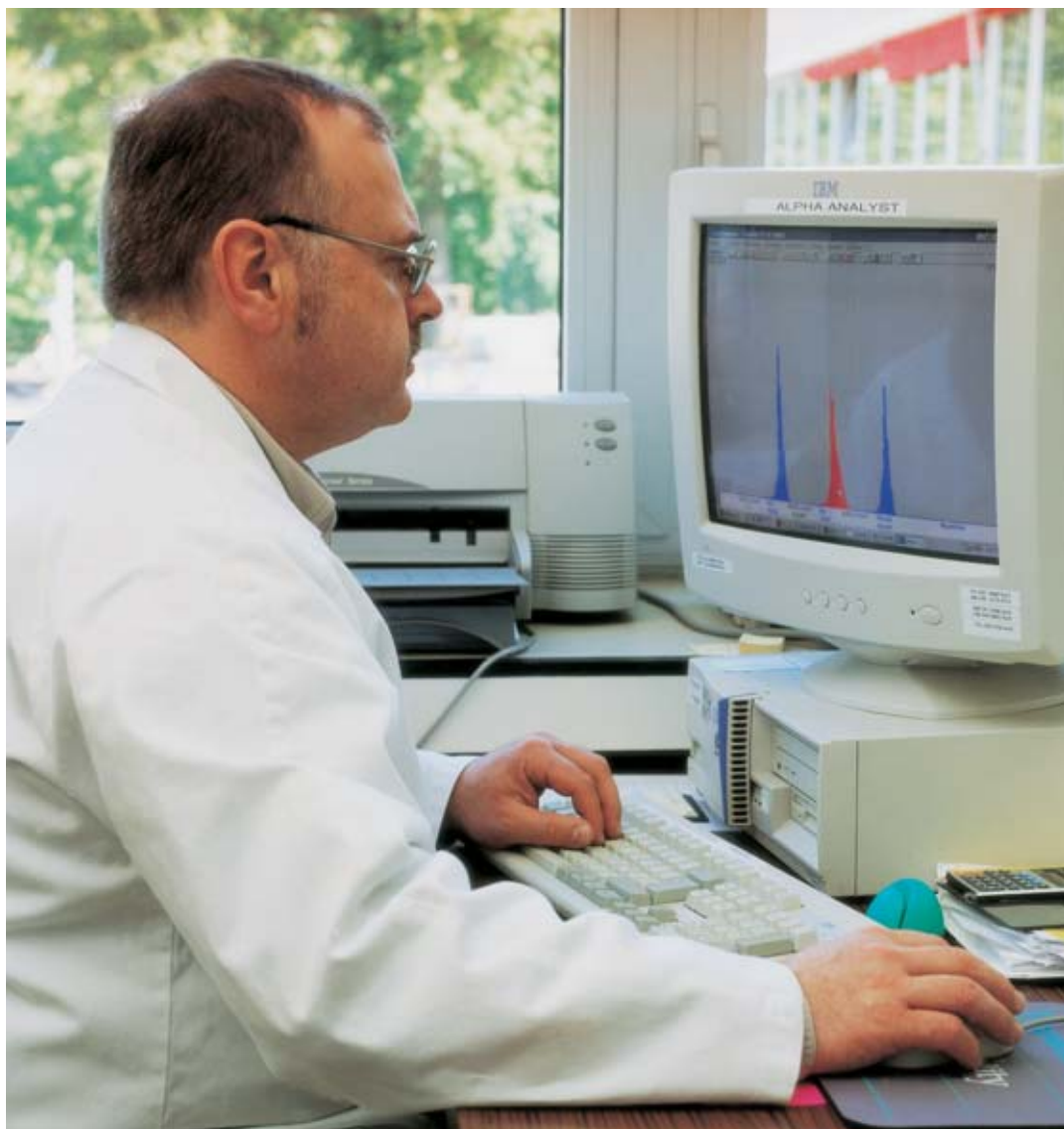
Alpha spectrometry evaluates exposure to toxic agents such as uranium and transuranics , via urine or faeces assay.
