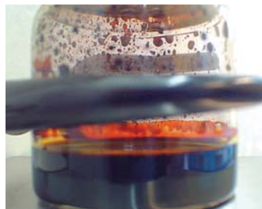
Bunsen reaction: separation of the two acids obtained in an experiment, carried out at CEA/Saclay, on thermochemical-cycle water splitting for hydrogen generation by the iodine-sulfur process.
