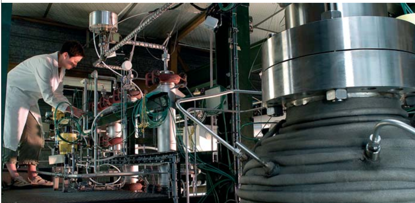
Analysis of product gases at the outlet of the experimental reactor set up at CEA/Grenoble for investigation of steam biomass gasification on a high-temperature (800-1,000 °C) fluidized bed, for the purposes of synthesis gas and biofuel production. This reactor allows characterization of efficiency, and to gain knowledge as to management and control of this type of device, and further allows testing of technological components (biomass feed and filtration).
