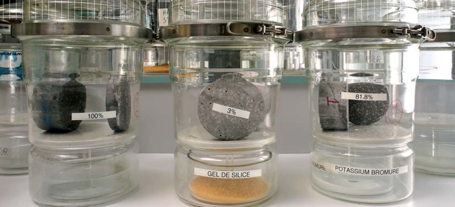
Desiccators for the preparation of concrete samples, before they are placed on the Banco test bench (investigation of chloride migration) and the Bandy test bench (measurement of hydrogen diffusion through the lid of an ILW-LL waste container), at CEA's Marcoule Center.
