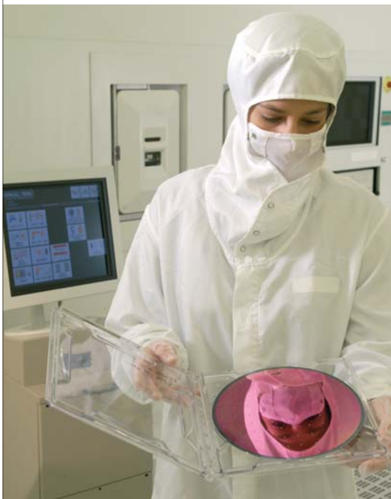
In a clean-room at the CEA Grenoble, a 200 mm diameter SOI wafer having undergone several technological steps, initially fabricated by the Smart Cut™ technology. Smart Cut™ is based on ion implantation (the machine can be seen in the background) and direct wafer bonding.
