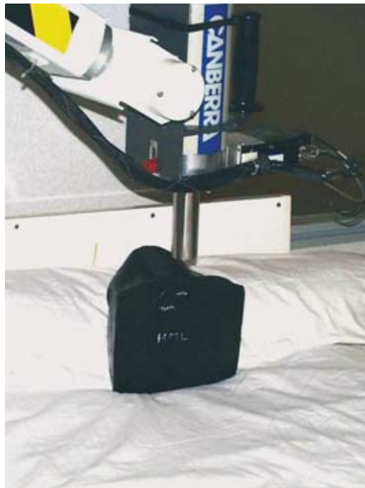
"Ghost" for the calibration of a thyroid irradiation detector at the medical service of Cogema Marcoule.
