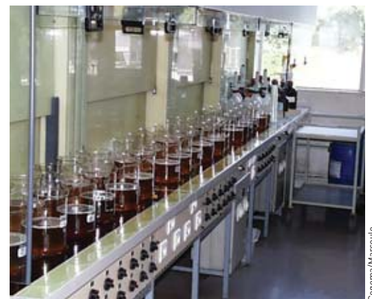
Testing for the presence of actinides in the urine of personnel during routine radiotoxicological analysis carried out by the medical analysis laboratory at CEA Marcoule.
