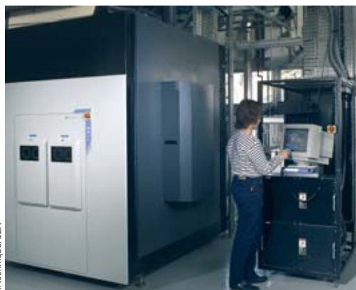
Centura reactor, installed at CEA Grenoble, dedicated to the large-scale growth of carbon nanotubes by the chemical vapour deposition (CVD) process.
