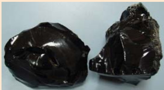
A volcanic glass (left) may be seen as a natural analog of nuclear glass of the R7T7 type (right).
