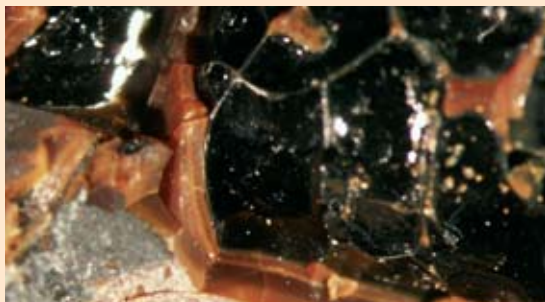
The alteration product of basaltic glasses, palagonite, is an analog of the alteration gel from borosilicate nuclear glasses.
