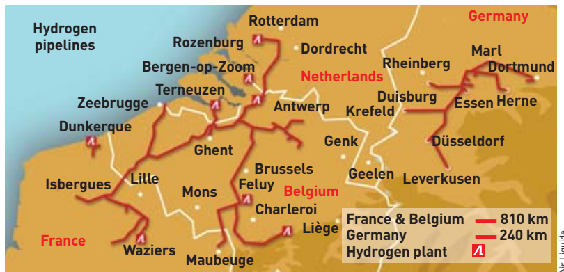
Figure. Air liquide's 100-bar gaseous-hydrogen supply pipeline grid covering France, Benelux and Germany.
